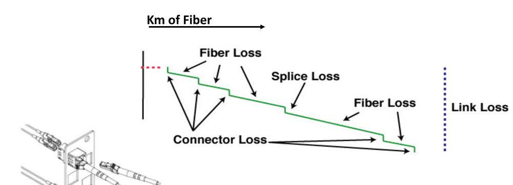
Patchloss from 0,3 to 5dB Depending on damage/dirt
