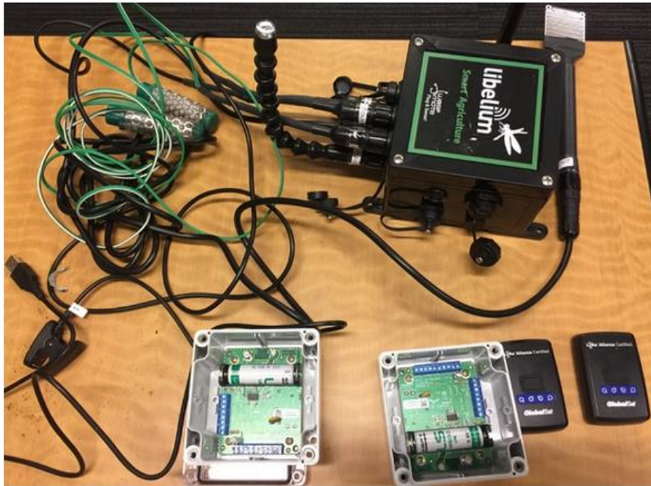
Photo 5: LoRaWAN sensors used by the City of Calgary
